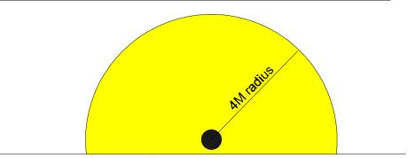
Sensor wall mounted in a corridoor showing limitation of sensing capability
