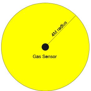
Perimeter representing 50 square meters as the sensors capable sensing zone
